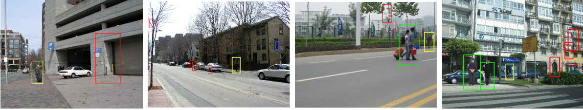
Figure 5.9: Negative results from using a HOG/SVM detector with MSR, positive results at 30% of WSR after non-max suppression. Yellow rectangles indicate FN caused by MSR (affecting performance); blue rectangles indicate avoided false positives (improving performance); TP are marked with green, while red rectangles are FP.
