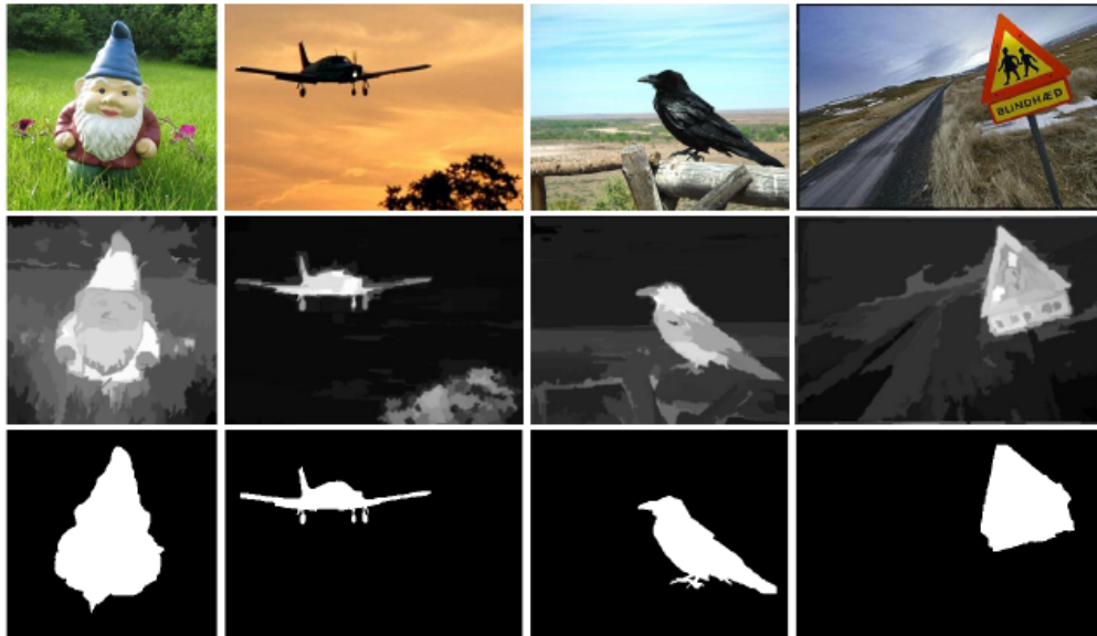
Figure 2.2: Examples of saliency detection and segmentation using [Cheng et al. 2011a]. In the second row the saliency maps generated from the input images from the first row. The third row are the object masks generated from the saliency map. Image taken from [Cheng et al. 2011a].
