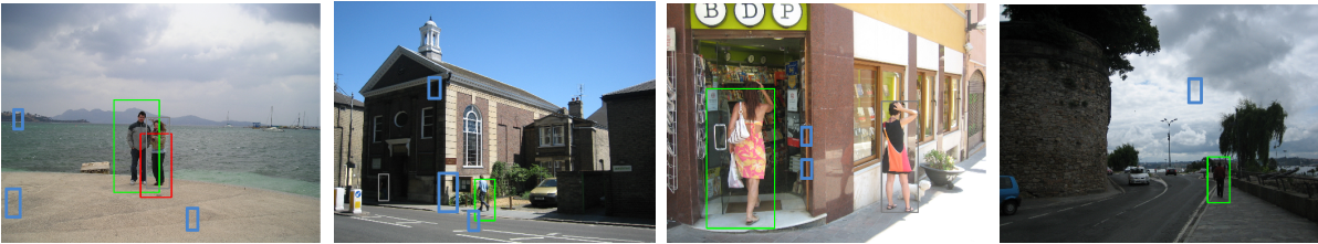
Figure 5.10: Positive results from using a Viola Jones detector with MSR, positive results at 30% of WSR after non-max suppression. Blue rectangles indicate avoided false positives (improving performance); TP are marked with green and FP with red.
